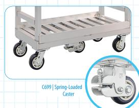
**Solution:** New Age Industrial offers a **five-wheel configuration** that includes four (4) swivel casters and one (1) rigid, spring-loaded caster in the center. This setup keeps the cart moving in a straight line until the operator wants to turn it. This center wheel also provides a zero-turn radius that keeps all five (5) wheels on the ground.
