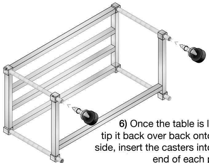
6) Once the table is level, tip it back over back onto the side, insert the casters into the end of each post.
